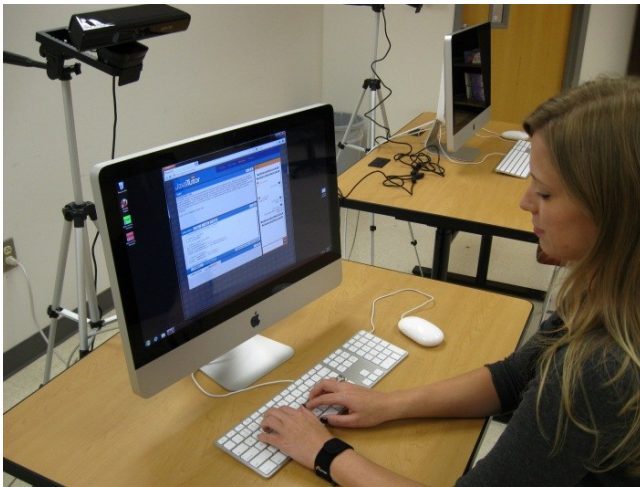
Figure 1. Student workstation with depth camera, skin conductance bracelet, and computer with webcam
