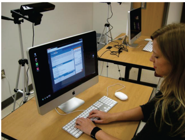
Figure 2: The workstation with Kinect depth-sensor, webcam and tutorial dialogue interface.
